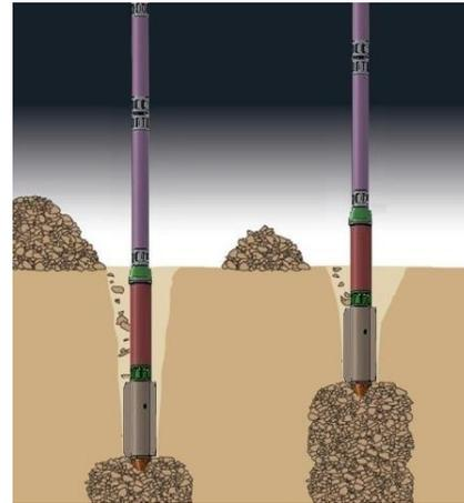
Vibroflotation reinforcement method
